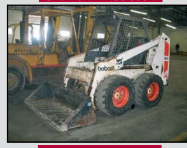
BOBCAT 843 SKID STEER LOADER
