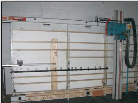
HOLZHER PANEL SAW
