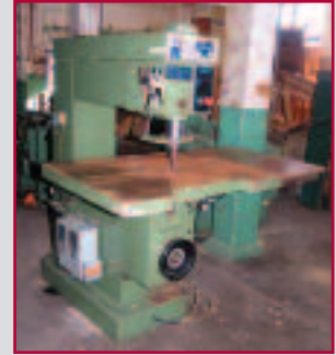
SAOM PIN ROUTER
