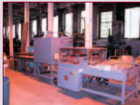
SHANKLIN SHRINK SEALER & TUNNEL
